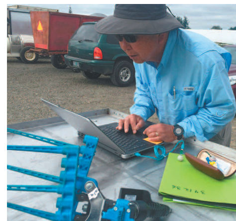
Dr. Fumi Takeda measuring blueberry bruise damage in the field with the BIRD sensor.
